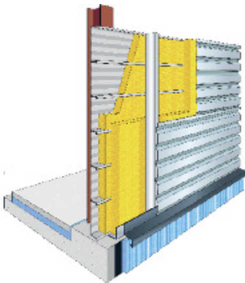
Metal cassette system for an exterior wall
