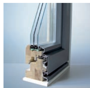
CLIMATOP® MAX – optimum thermal insulation ( U = 0.5 \text{ W}/\text{m}^2\text{K} ) and maximum utilization of solar radiation in winter ( g = 0.6 )
